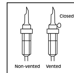
3. Use a non-vented infusion set or close the air vent on a vented set. Follow the instructions for use for the infusion set. Use a spike with diameter of 5.6 +/- 0.1 mm.
