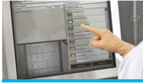
Electronic dose queue allows users to identify orders by type and urgency
